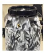
Screw in the adapter using a wrench, making sure to protect the threads and place in lock nut. Use pliers to tighten, making sure to cover threads with a rag or pipe cap to prevent damage.
