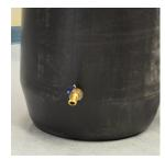
Next, crawl inside your barrel to seal the faucet. Press rubber gasket tightly against faucet/barrel wall, follow with big washer (indented side towards barrel) and screw on lock nut. Tighten lock nut with pliers. Using a flashlight is helpful. The faucet is now connected.
